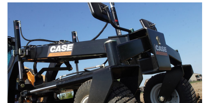
Optional twin convex mirrors give the operator visibility down to the moldboard corners
